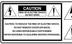
This symbol warns the user that uninsulated voltage within the unit may have sufficient magnitude to cause electric shock. Therefore, it is dangerous to make any kind of contact with any inside part of this unit.
